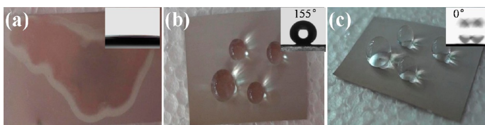
Figure 7. (a) Unmodified HAPOP surface shows superhydrophilicity with a WCA of 3^\circ . (b) Top photograph of the water droplets on the PDES-MS surface. The inset indicates that the surface could obtain a WCA of 155^\circ . (c) Side-view photograph of the water droplets. The inset shows that the surface presents a sliding behavior with an extremely low SA of 0^\circ .
